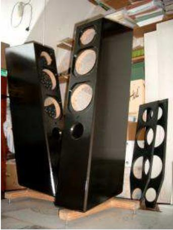
*The T-shaped wooden foot and in the background the panels for the speaker grille.*
