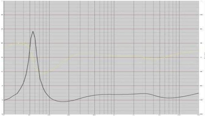
The impedance curve for a closed box simulation. The main horizontal division is 4 ohms with sub divisions of 1 ohms +/- 1 ohm over the whole range except for the bass impedance peak (the reflex will show two peaks).
