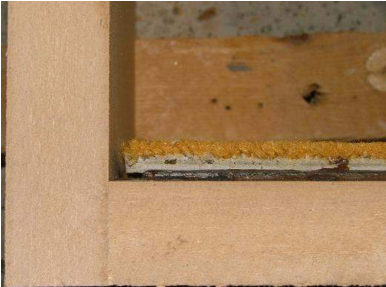
Mdf + high-mass damping sheet + carpet tile
