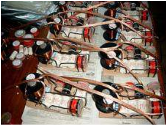
The crossovers during assembly.
