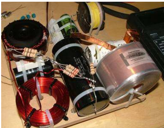
crossovers with the separate LCR network mounted on the back panel.
