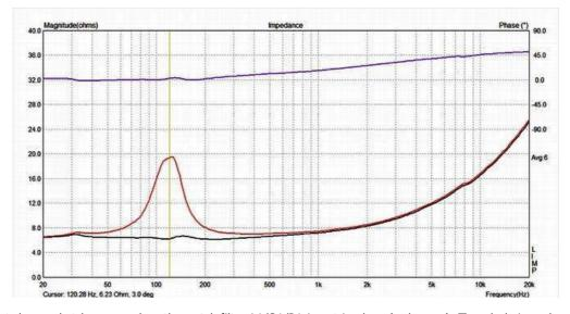
The second plot shows what happens when the notch filter L1/C1/R1 is put in place (red curve). The whole impedance from 100Hz to 10kHz is raised, the loudspeaker will therefore produce less energy in this region. The bass and top octave will thus be let through unaltered. When the last two correction networks are added you get the black curve: a ruler flat impedance of 12 ohms
