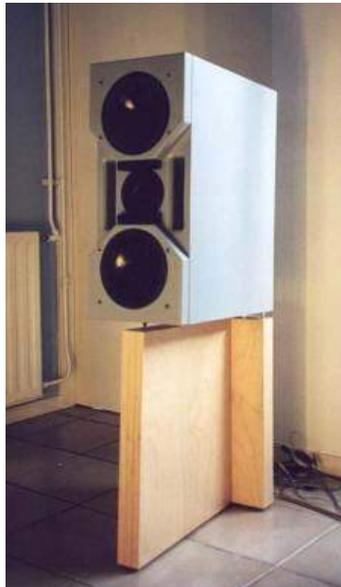
An exercise in trying to use the series network for two different configurations using the same loudspeakers. The guinea pig is a classic MTM configuration using two Seas 7-inch mid-woofers and a 1-inch soft dome tweeter in a stand mounted symmetrical reflex loaded cabinet. Furthermore the drivers are physically time aligned.
