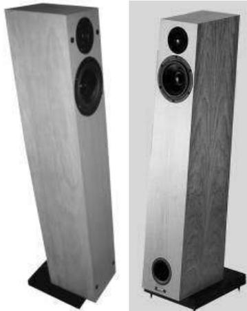
One thing missing on the Humble Homemade Hifi site up to now: a standard 2-way floorstander. This configuration uses a Vifa 7-inch mid-woofer and a Seas 1-inch soft dome tweeter in a reflex loaded floor standing cabinet. Furthermore the drivers are physically time aligned.
