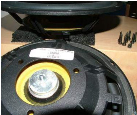
Note the washers attached to the rear of the SP21R.
