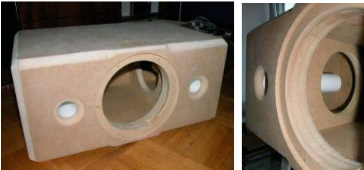
Note the internal partition with its circular cutout.
