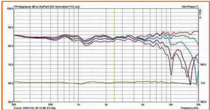
Above left: individual frequency curves of the midwoofer (blue) and tweeter (green) and the summed response of the finished system (red) with corresponding acoustic minimum phase; frequency range 200Hz - 20kHz; horizontal range 50dB - 100dB, subdivision 2dB's.
