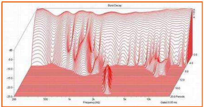
Above left: cumulative spectral decay of the finished system; frequency range 200Hz - 20kHz; horizontal range -25dB, time window 4,49ms.
