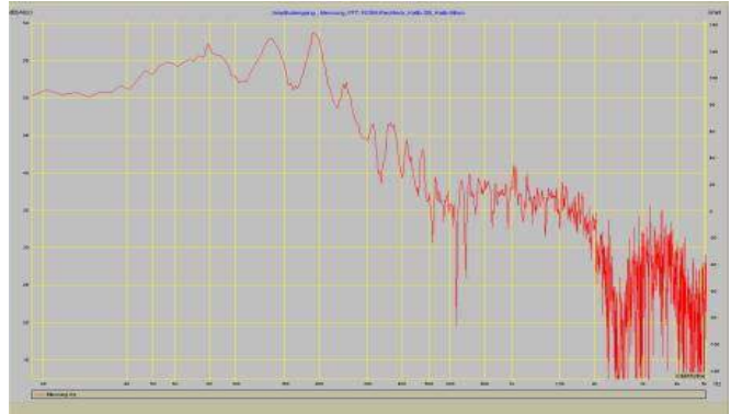
waterfall-spectrum finished speaker 3ms/-30dB; nearfield output from port, scale 5dB / 20-2000Hz
